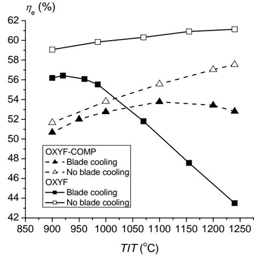
Fig. 8 The power generation efficiency  $\eta_e$  vs.  $TIT$
