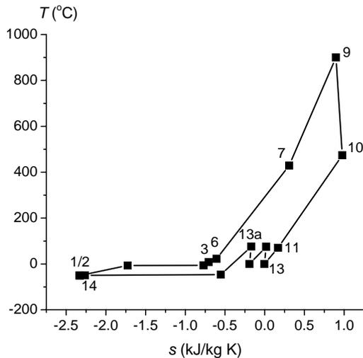
Fig.2 Cycle  $T$ - $s$  diagram in the OXYF-COMP system
