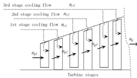
Fig. A1 Schematic diagram of the turbine air cooling model
