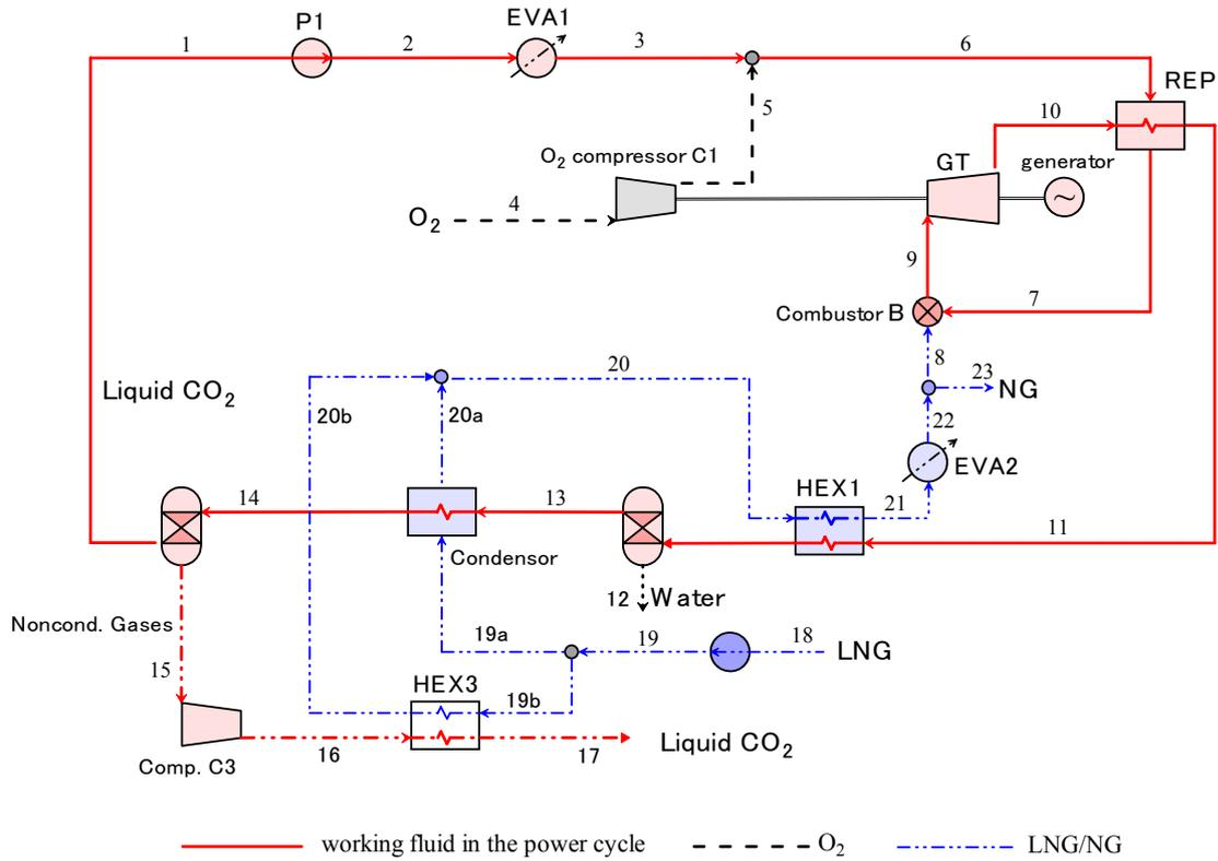
Fig. 3 The process flowsheet of the OXYF system
