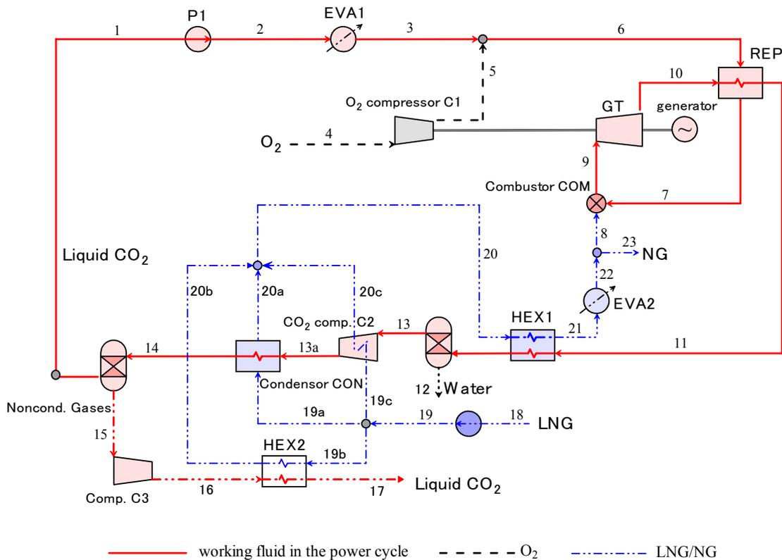
Fig. 1 The process flowsheet of the OXYF-COMP system
