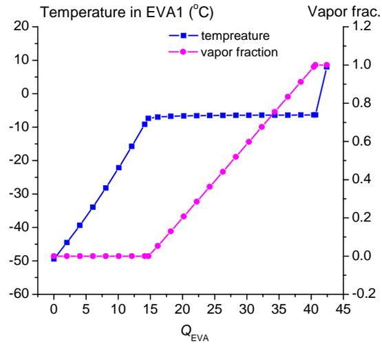
Fig 14 The temperature profile of the produced refrigeration in EVA1 in the OXYF system
