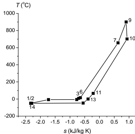
Fig.4 Cycle T-s diagram in the OXYF system
