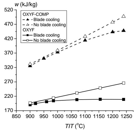
Fig.5 The specific power output  $w$  vs.  $TIT$
