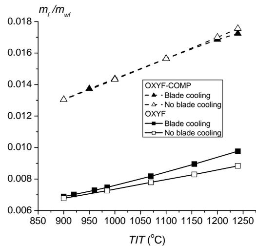
Fig.6 The fuel mass flow rate  $m_f$  vs.  $TIT$
