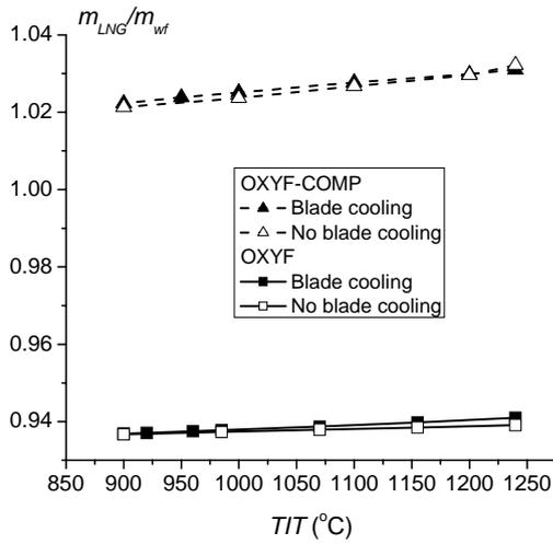
Fig. 7 The evaporated LNG mass flow rate vs.  $TIT$
